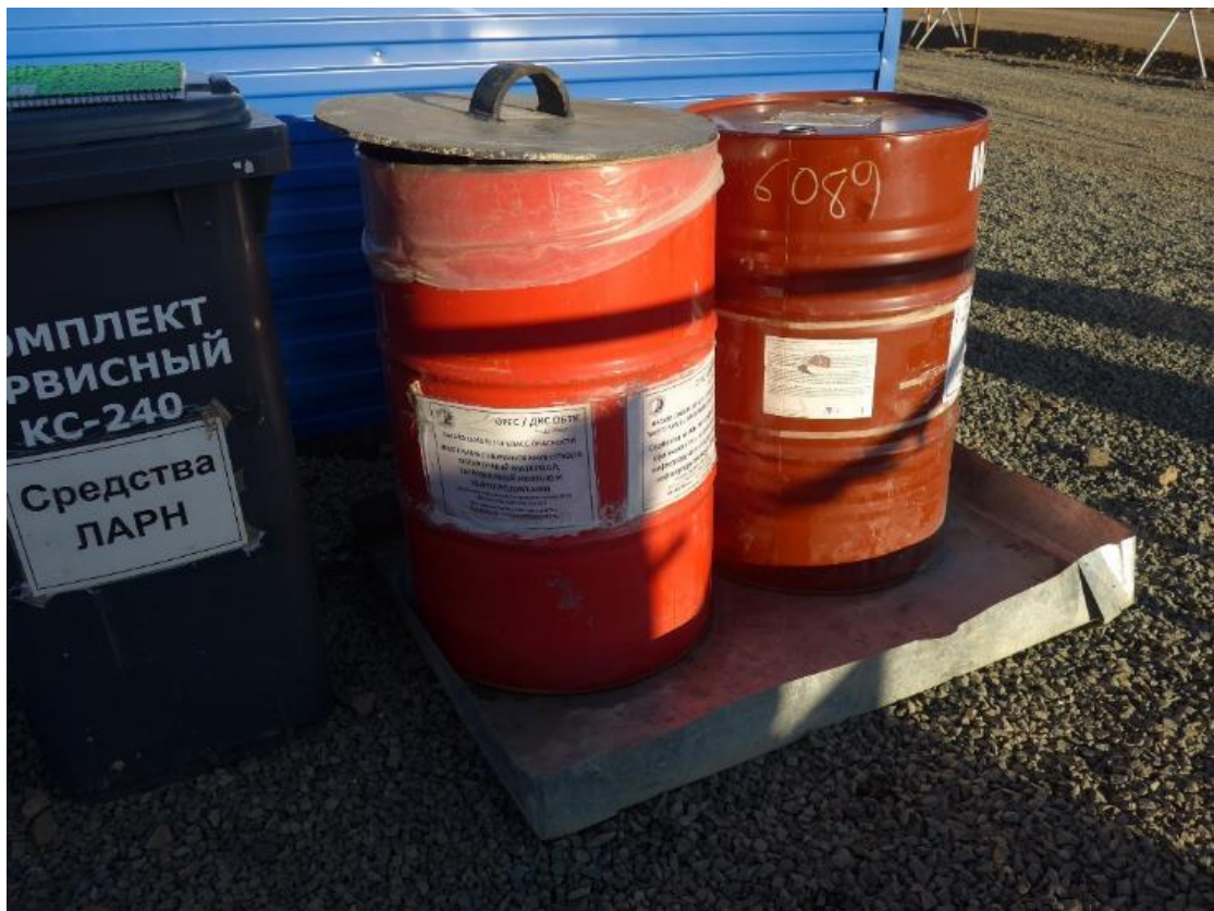
Photo 27 – Clearly labelled waste oil / oily rags storage containers
