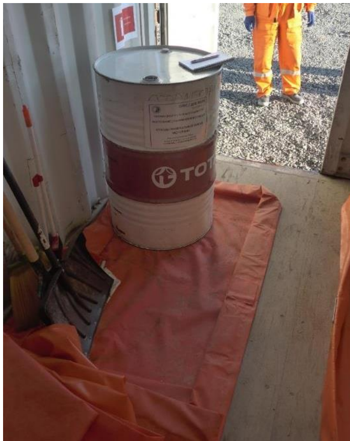
Photo 24 – Fully collapsed portable bund around a waste oil drum
