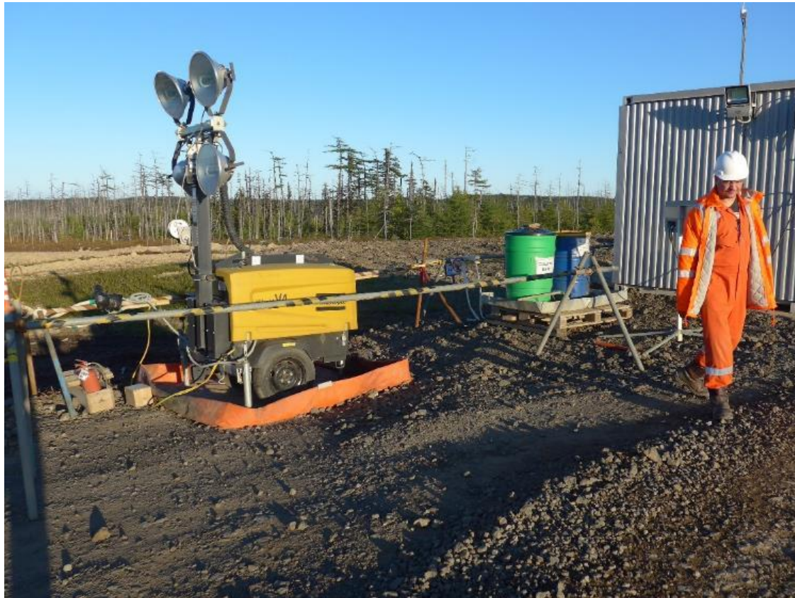
Photo 22 – Example of secondary containment for a generator and oil drums
