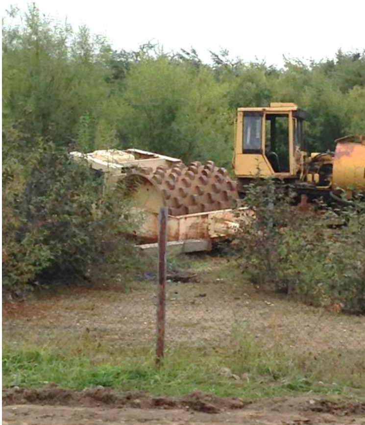
Photo 17 - Non-operational studded roller - to be replaced
