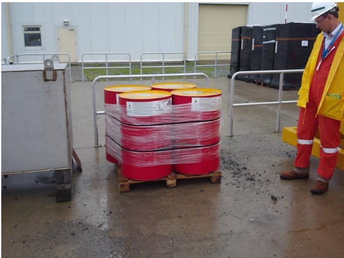
Photo 10 – Four drums of oil with no secondary containment
